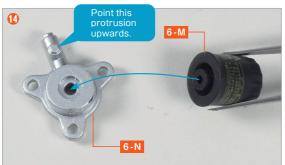
Align the screw hole on the back of the Oil Filter 6-M with the screw hole on the Oil Filter Bracket 6-N.
