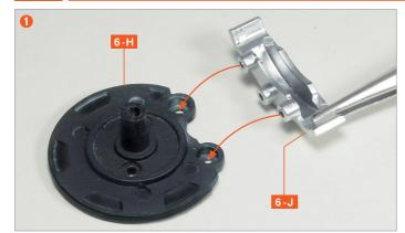
Align the protrusions on the **Brake Caliper (2) 6-J** with the two holes on the **Brake Disc Dust Cover 6-H**.
