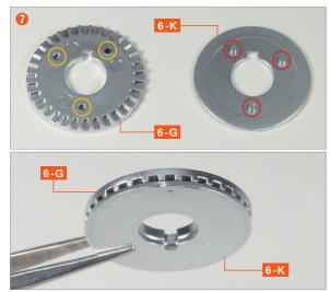
Align the three pins and holes of **Brake Disc (1) 6-G** and **Brake Disc (2) 6-K**, and fit them together.
