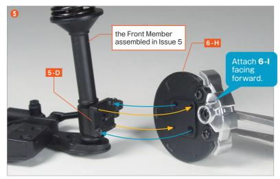
Prepare the **Front Member** assembled in Issue 5, and combine the **Knuckle Arm (L) 5-D** with **6-H**.
