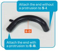
Make sure the orientation is correct, then fit the Water Outlet Pipe 6-D into 6-B and the Water Bypass Pipe (2) 5-I.
