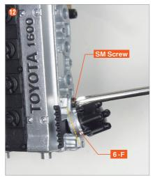
**6-F** is angled, but tighten the **SM screw** vertically into **3-G**. First, secure one side to set the mounting position.
